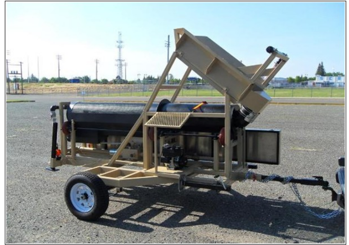
Not shown is a removable 4' long discharge chute that is adjustable in angle and stows for transport.
